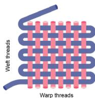
A simple cotton cloth where the warp and weft pass over and under each other forming a criss-cross pattern. Calico (muslin) is naturally grey and can be soft or coarse.
