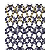
A single yarn creates interlocking loops across the fabric. If a loop breaks, a hole forms and ladders. Made by hand or machine.
