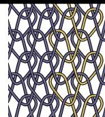
Formed by vertical loops like a series of chains. It can only be produced on a machine.
