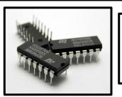
A dual in line (DIL) package which means it has a rectangular housing and two parallel rows of electrical connecting pins.
